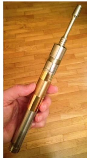
**Tube Mod** – Any PV or APV that comes in a tube shape. Most sizes are about 6-8 inches, but they can be longer.
