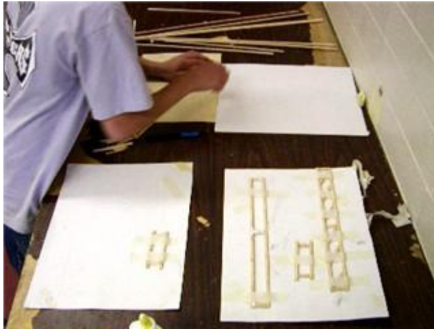
Gluing the substructure and cross trusses together.
