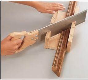
**REAL LIFE MITER BOX** This box has slotted sides to guide a saw when making angled cuts.
