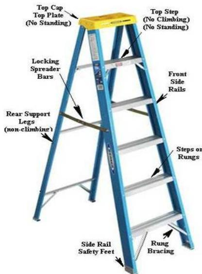
even surface. If the ground is too soft there is a possibility of sinking and shifting the ladder which can throw you off balance. If you are working on a tall ladder, consider barricading off the area to prevent pedestrians from walking beneath the ladder. This will also prevent you from injuring someone if you accidentally drop something as a pedestrian is walking by.
