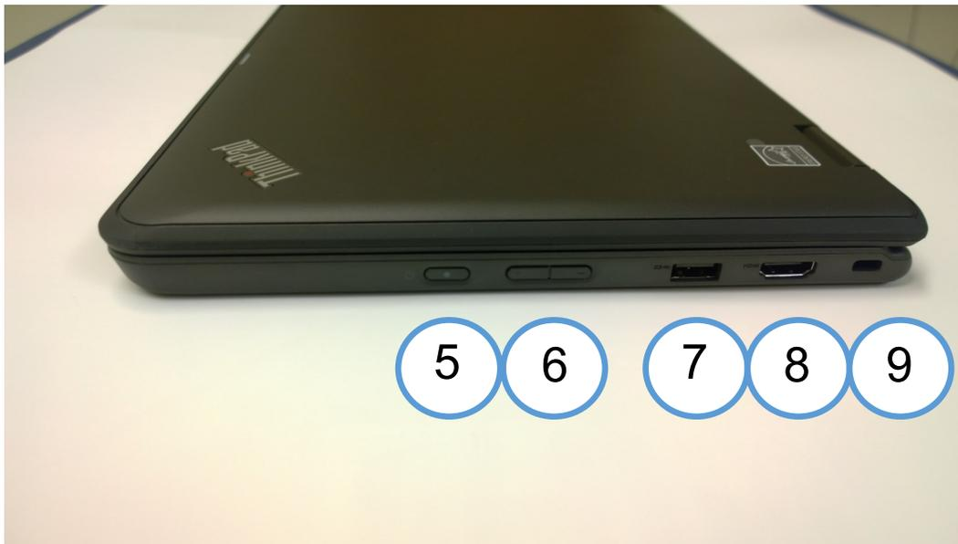
5. Power Button: The power button turns the device on and off. The bulk of troubleshooting starts and ends at this button. Most Wi-Fi, trackpad, and other issues can be solved by holding the power button until the machine turns off, then pressing the button to turn it back on.
