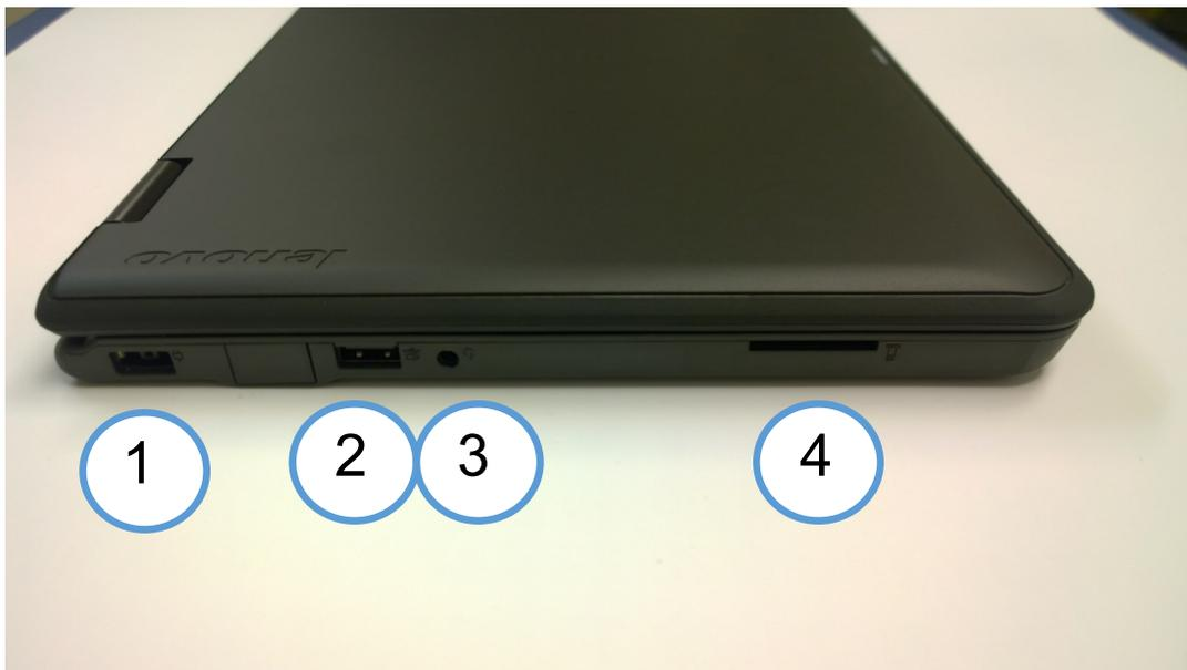
1. Charge Port: Chromebooks supplied by RBHS should only be used with an RBHS supplied power adapter. Replacements are available in the bookstore at a charge.
